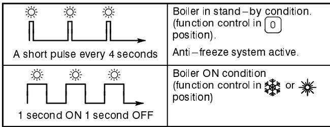
Boiler in stand-by condition. (function control in 0 position).
