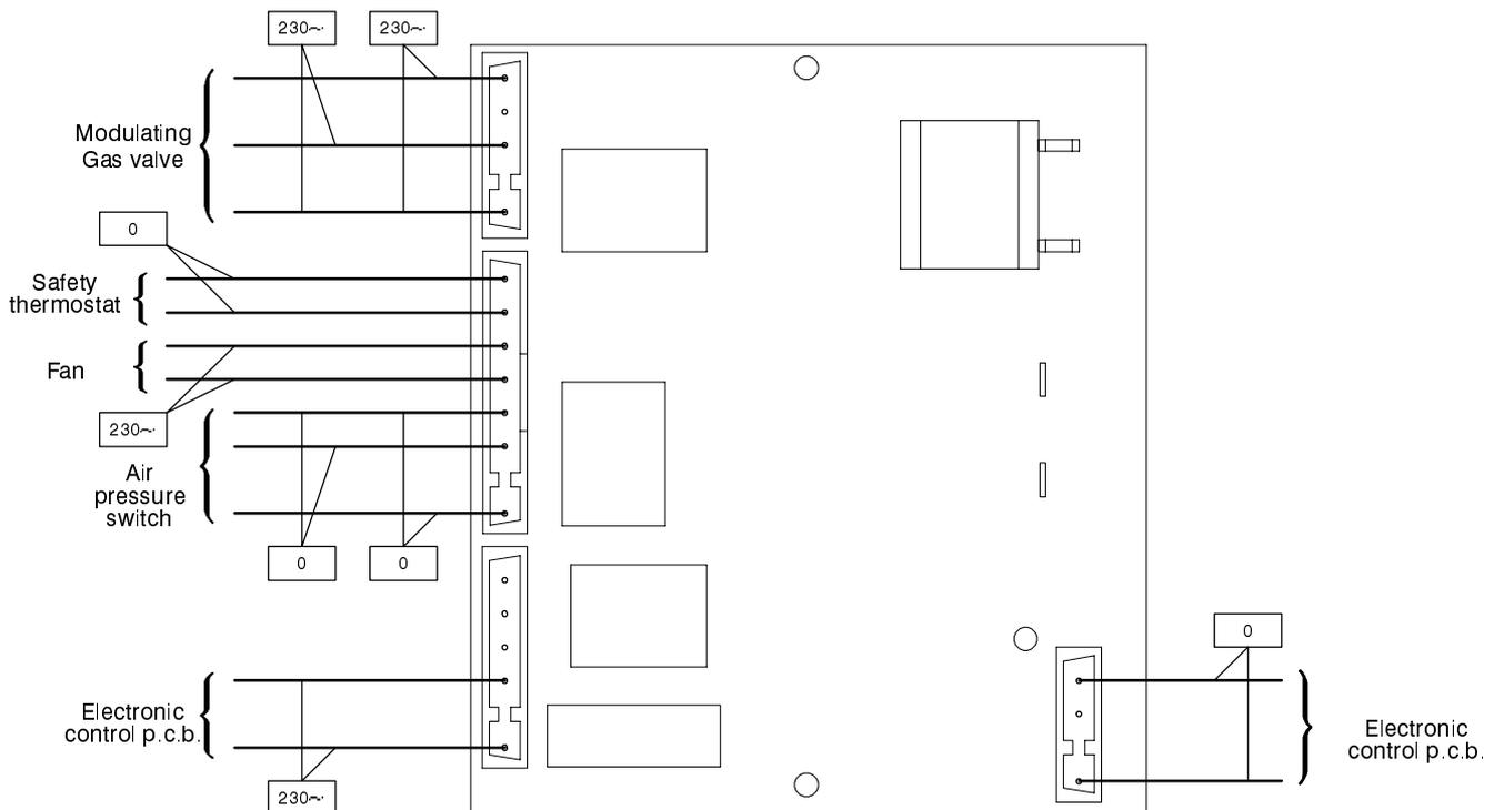
**Diagrams for boiler equipped with full sequence ignition device type: Honeywell FPLD**
