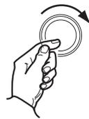
**STEP 3** - Press the Dial Knob again and the On Off mode will flash. While flashing turn the Dial to toggle between On and Off. Press Dial to select.
