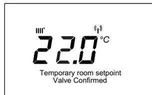
**STEP 1** - Turn the Dial Knob and the temperature will appear. Turn the Dial Knob again and whilst flashing keep turning the dial to display the required temperature.
