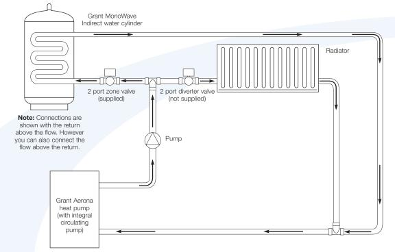
Figure 5-2: 'S' Plan system schematic - for Grant Aerona heat pump
