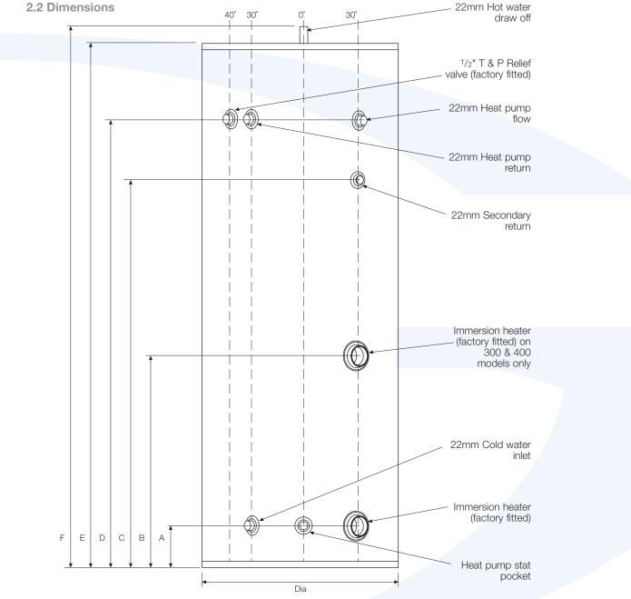
Figure 2-2: MonoWave HP indirect cylinder dimensions
