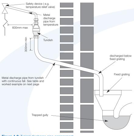
Figure 4-2: Typical discharge pipe arrangement
