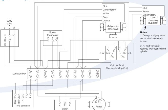
Figure 5-5: 'Y' Plan wiring layout
