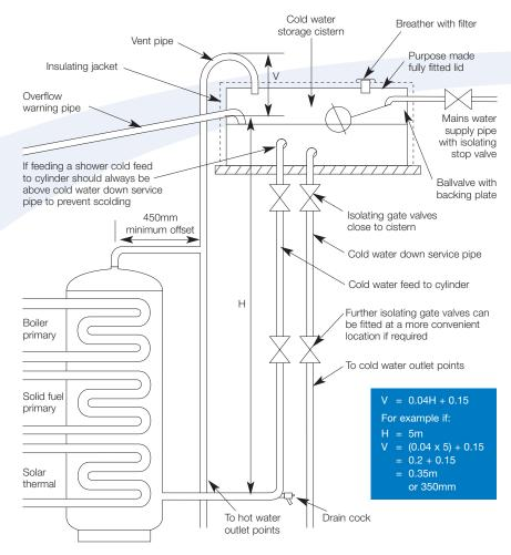
Figure4-1: Open vented cylinder
