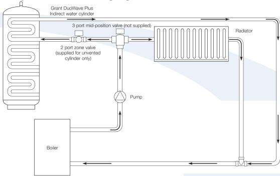
Figure 5-4: 'Y' Plan system schematic
