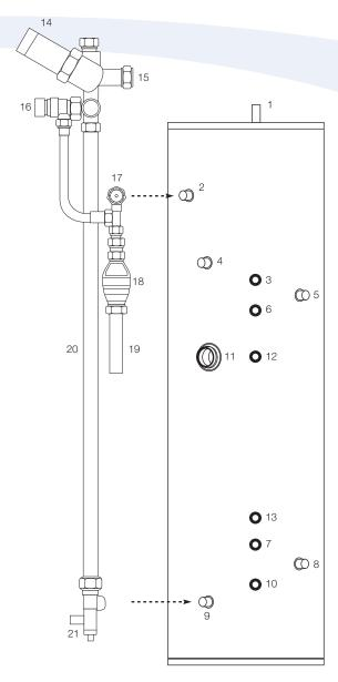
Figure 2-2: Cylinder connections and controls
