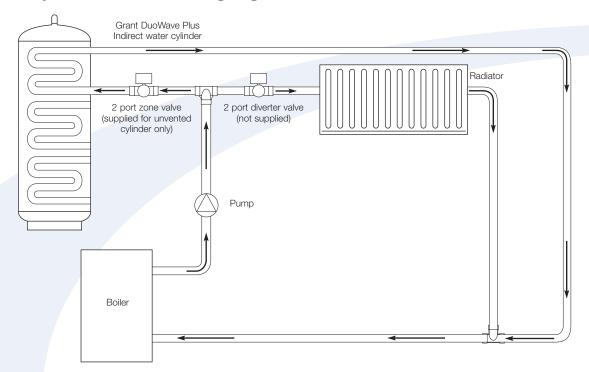
Figure 5-6: 'S' Plan system schematic
