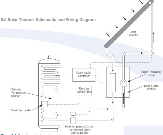
Figure 5-8: Solar thermal schematic
