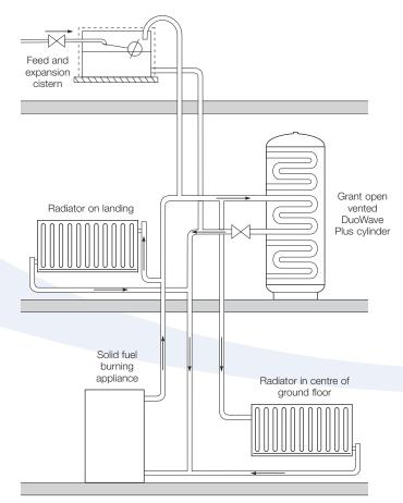
Figure 3-1: Typical installation of an uncontrolled appliance
