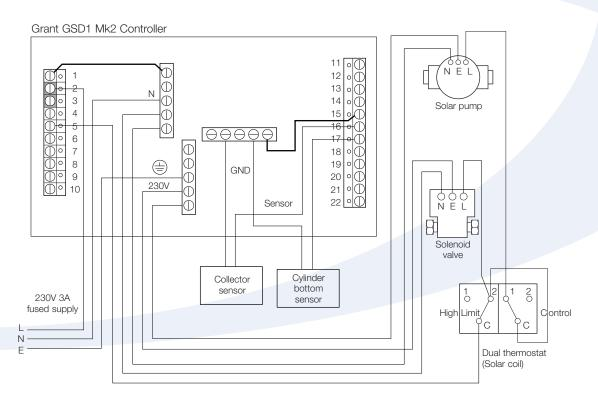
Figure 5-9: Solar thermal system typical hydraulic wiring layout
