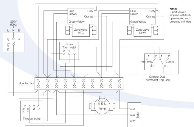
Figure 5-7: 'S' Plan wiring layout
