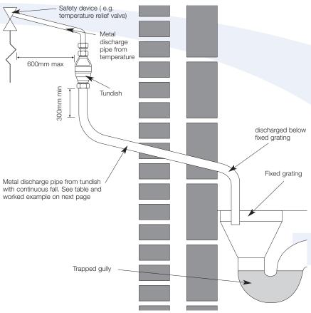
Figure 4-2: Typical discharge pipe arrangement
