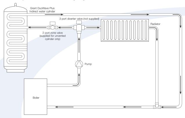
Figure 5-2: 'W' Plan system schematic
