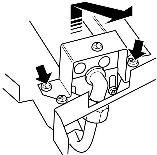
Figure 49. Removal of burner
