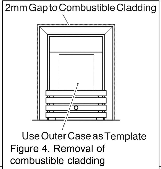
100mm minimum mandatory clearance to combustible surfaces projecting beyond front of appliance. For access purposes a 10mm clearance is recommended to non-combustible surfaces
