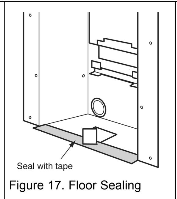
Figure 17. Floor Sealing
