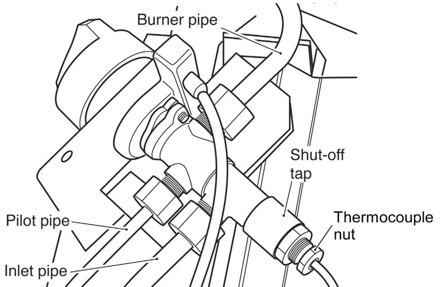
Figure 48. Gas valve (Viewed from rear with burner turned over)
