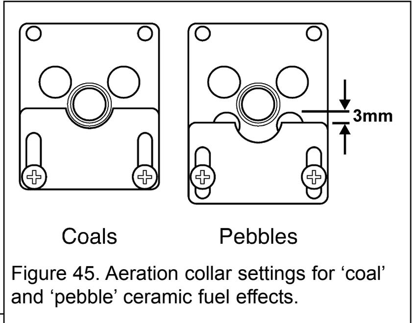
Figure 45. Aeration collar settings for 'coal' and 'pebble' ceramic fuel effects.
