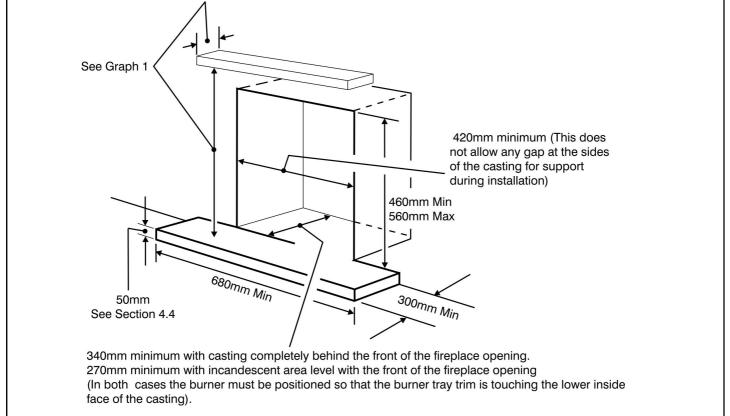
Figure 2. Hearth and fireplace opening for installations using the **SPANISH BASKET CASTING ONLY**
