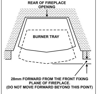
Figure 5. Burner positioning
