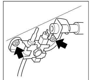
Figure 24. Pilot unit removal
