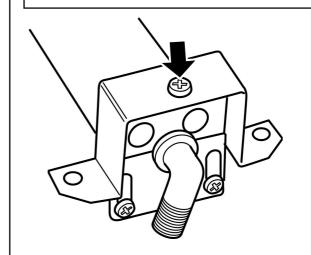
Figure 27. Main burner Injector removal
