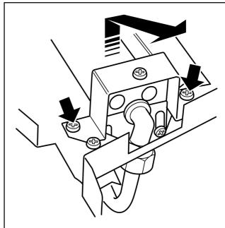
Figure 26. Removal of burner
