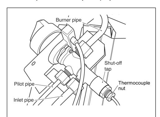
Figure 25. Gas valve (Viewed from rear with burner turned over and front leg bracket removed)
