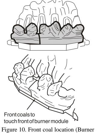
Figure 10. Front coal location (Burner tray design may differ from that shown)
