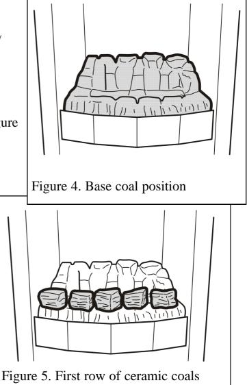
be evenly spaced. Rest them on the ledges above the slots in the base coal (See figure 7).
