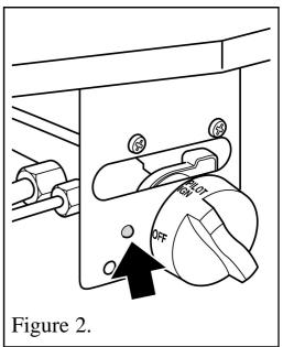
• Once the pilot light is established, the main burner can be lit by depressing and turning the control knob anticlockwise to the "**High**" position.
