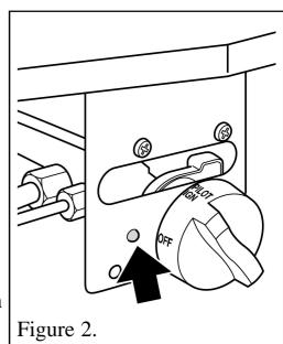
• If the pilot does not ignite instantly, repeat procedure. If after 10 seconds pilot ignition has not occurred, turn the control knob back to the "Off" position, wait for 3 minutes and then repeat the ignition procedure.
