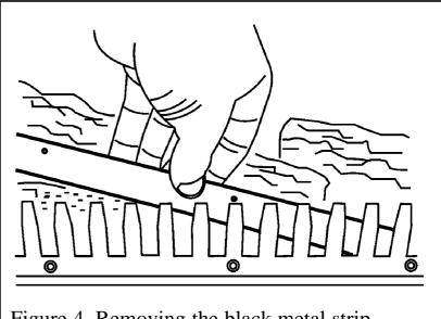
Figure 4. Removing the black metal strip
