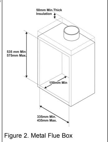
The current revision of the standard requires 16,500mm<sup>2</sup>. This appliance is suitable in both cases. The total depth of the opening measured from the finished front of the fireplace (Including plaster, surround etc.) must be *not less than 120mm*. See figure 3. The current versions of BS1289 and BS EN 1806 recommend that there should be an air space or insulation between the flue blocks and the plaster because heat transfer may
