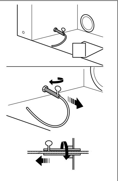
Figure 16. Lower Cable Retention
