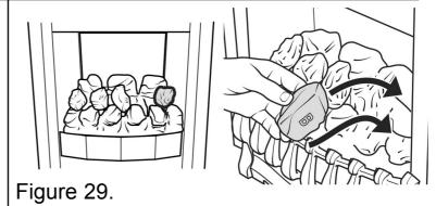
7. Place the remaining type "A" coal between the front and rear base coals. The letter "A" should be upside down with its rear face between the right and centre coals of the rear base coal. Angle the coal so that the gap between it and the type "B" coal to its right is appreciably larger than the gap between it and the type "A" coal to its left but do not have it touching the
