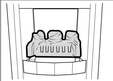
Figure 24. Rear Base Coal Position
