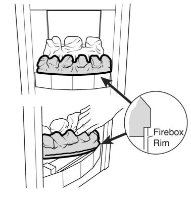
Figure 25. Front base coal position
