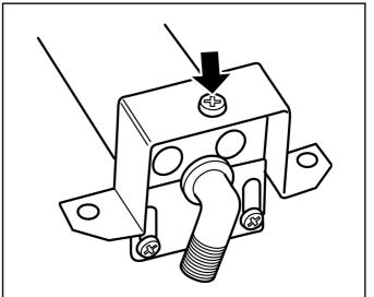
Figure 50. Main burner Injector removal
