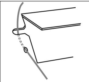
Figure 14. Upper cable retention
