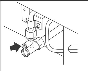
Figure 18. Pressure test point
