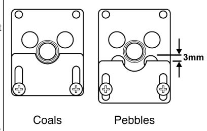
Figure 45. Aeration collar settings for 'coal' and 'pebble' ceramic fuel effects.
