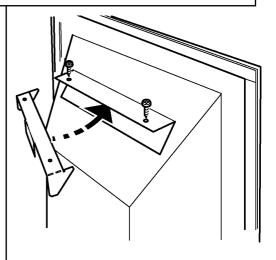
Figure 12. Fixing restrictor
