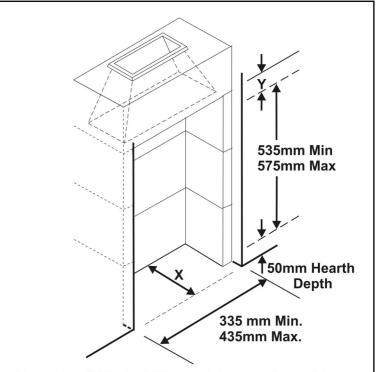
Dimension 'X' to be 120mm minimum. This will be made up of 115mm starter block depth plus at least 5mm of non-combustible fireplace material (Plaster, marble, etc).
