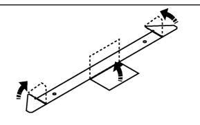
Figure 11. Bending the restrictor
