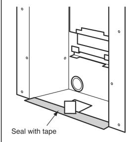
Figure 17. Floor Sealing
