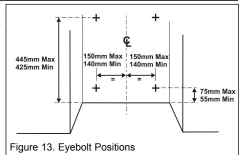
figure 13 using a no.12 masonry drill. The holes should be equidistant each side of the centre line of the fireplace to ensure that the appliance finishes centrally in the opening when tension is applied to the cables.
