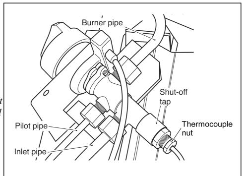
Figure 48. Gas valve (Viewed from rear with burner turned over)
