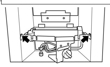
Figure 46. Burner attachment points
