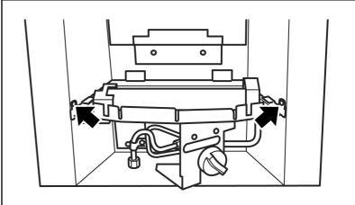
Figure 8. Burner attachment points
