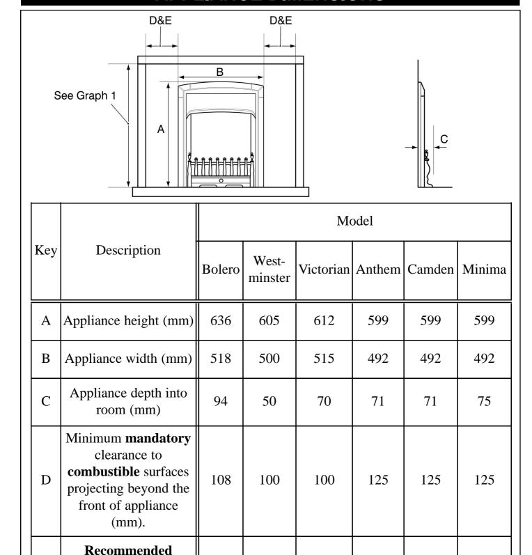
Figure 5. Appliance dimensions and clearances
