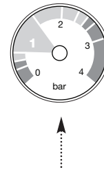
System Pressure Gauge
