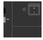
With the solar main switch on the Control Tower the solar circuit can be switched on or off. Switching off the solar circuit can be necessary in case of maintenance activities by your installer. This switch
