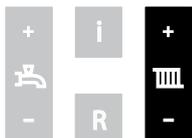
CH program OFF: Press – until the lowest value is reached and then press – again. The display is showing -- and the upper ◀ is off.
