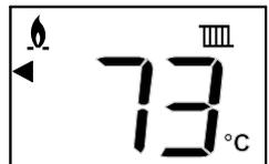
Standard view with device in operation for CH
