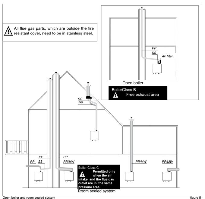
Open boiler and room sealed system
