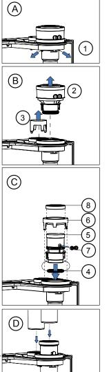
boiler conversion from concentric to parallel figure 6
