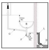
Terminate as close to the ground or drain as possible (below the grating and above the water level) while still allowing for safe dispersal of the condensate. Connection of a condensate drainage pipe to a drain may be subject to local building controls.
