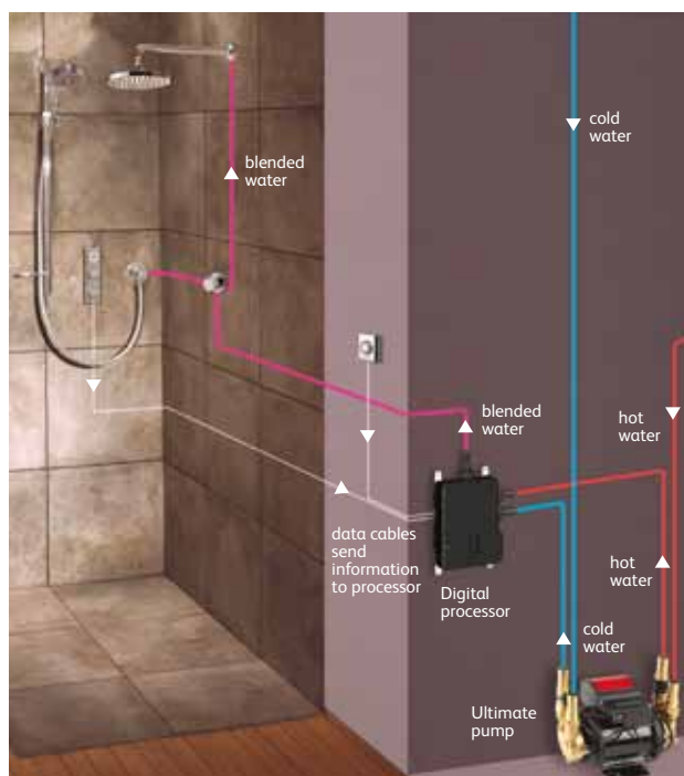
HiQu Digital concealed multiple outlet configuration with Ultimate 340 pump (suitable for Gravity water systems)
