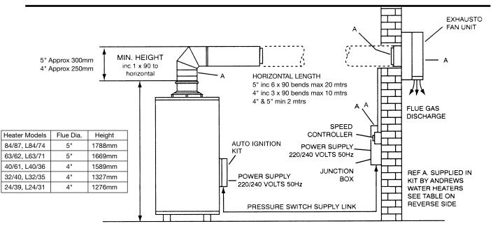
The Exhausto Flue Fan when used on Standard Range Water Heaters with the Solenoid Control Kit will give the following control
