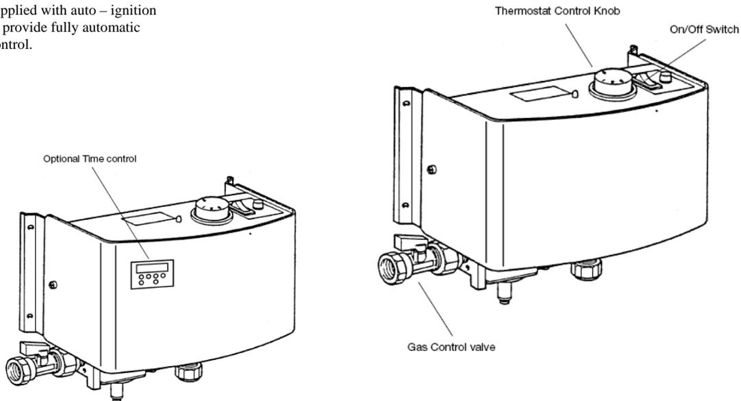
THE STANDARD RANGE AND RSC WATER HEATERS CAN BE SUPPLIED FOR PERMANENT PILOT OPERATION WITH THERMOCOUPLE ENERGISING TO OPEN THE MAIN BURNER VALVE. (No electricity supply required).
