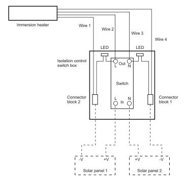
Note: Immersion heater wires are labelled 1 to 4.
