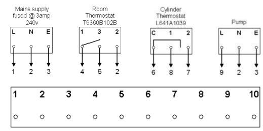
NOTE: Pump live must always be connected to the pump live terminal provided in the boiler control panel, e.g via junction box terminal 9
