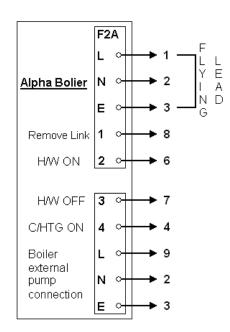
NOTE: To connect external control, remove link from terminals 1 and 2 and connect a 230/240v switched live to terminal 1
