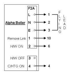
**NOTE:** To connect external control, remove link from terminals 1 and 2 and connect a 230/240v switched live to terminal 1
