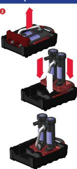
Lift the canisters from the base and slot into recessed area.
