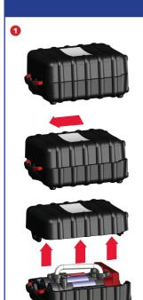
Lift the handle to unlock the box, slide and lift off the top case.
