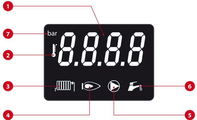
1. Numerical field displaying the temperatures
