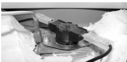
Fig. 26: Safety thermostat reset button.
