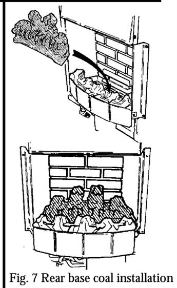
Fig. 7 Rear base coal installation
