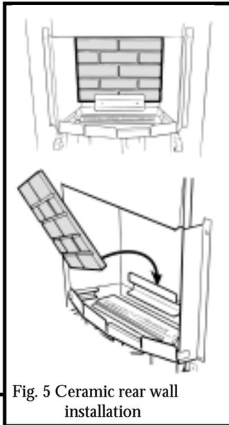
Fig. 5 Ceramic rear wall installation
