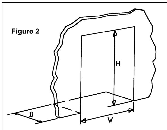
Remove any firebrick back and existing heating appliance. Examine the general condition of the builders opening and repair if necessary. Check dimensions of builders opening and if necessary, modify to those shown in Fig 2.
