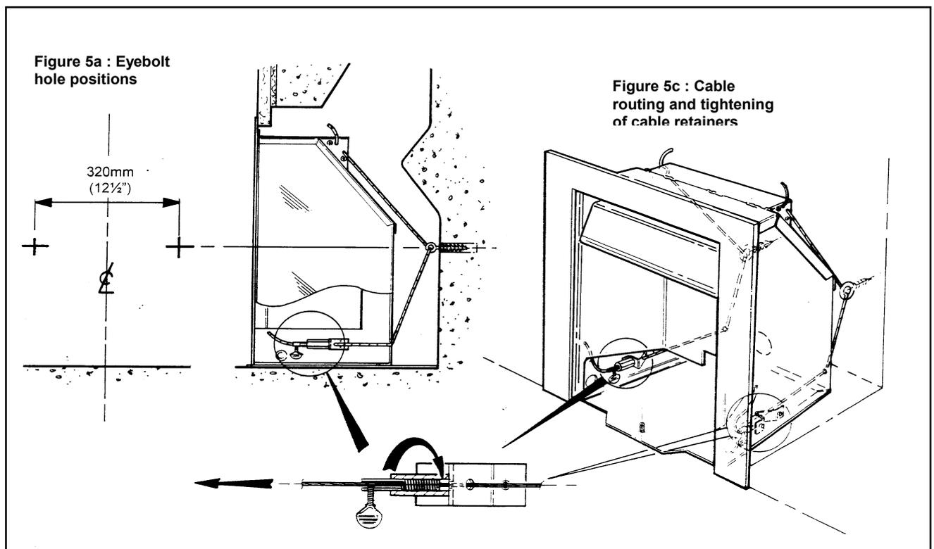
Figure 5a : Eyebolt hole positions
