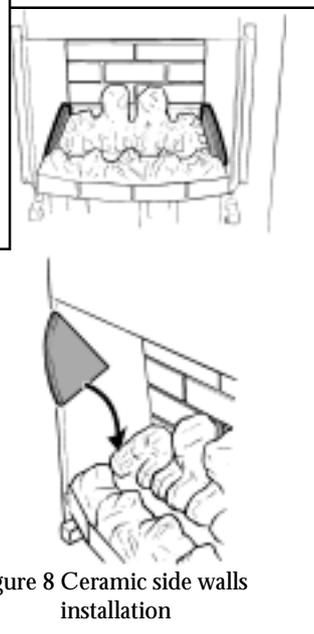
Figure 8 Ceramic side walls installation
