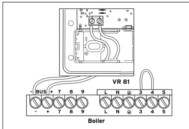
**Fig. 9.2 Electrical connection**
