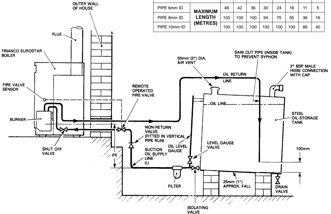
**FIG. 13 TWO PIPE OIL SUPPLY**
