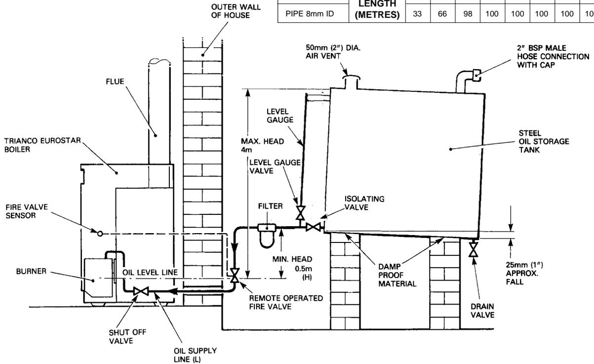
**FIG. 12 SINGLE PIPE OIL SUPPLY**
