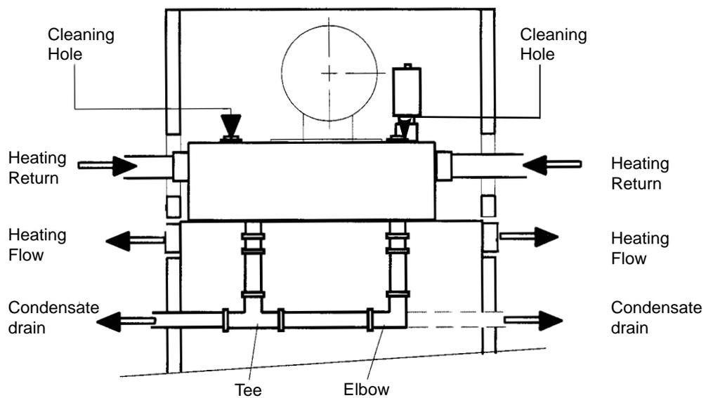
View of rear of boiler showing boiler connections. Connections can be made on L/H side or R/H side of boiler.
