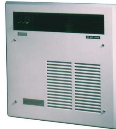
This heater appliance is intended for use as an air heater and is to be mounted recessed into an internal wall. It is to be mounted with the bottom edge between 100 mm and 1000 mm from the floor. Alternatively, it can be adapted for mounting on the wall by using a Smith's Surface Mounting Kit, which is supplied along with full instruction within this booklet.
