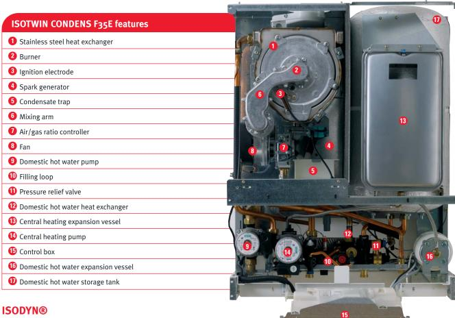
The ISOTWIN CONDENS uses a shift load storage principle to deliver up to 200 litres of usable domestic hot water. This is achieved by mixing water stored in the integral tank with water produced during normal domestic hot water operation. This is enough water to satisfy even the largest demands and once the tank has been depleted the ISOTWIN continues operate to in normal combi mode producing 14 l/min of hot water @ 35°C rise.
