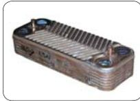
However, relatively small quantities of iron oxide (rust) can block the waterways, causing the boiler to cut out when in hot water mode. As little as 12 gm of rust can cause a heat exchanger to fail. A central heating system may contain several kg of loose rust, and therefore failures are common.
