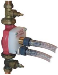
The CPII™ adaptor has been developed for use with heating system power flushing pumps, to enable them to be connected directly onto the body of standard heating system circulator pumps, after removal of the motor head.
