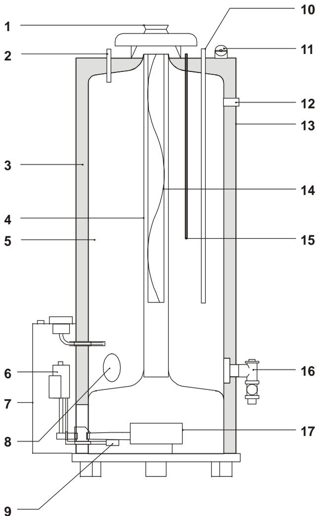
Figure 1 - Cross section of the heater
