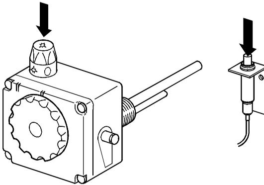
Drawing 6 - Operation of the gas control block
