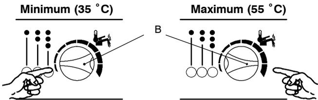
Adjustment of the DHW temperature is completely separate from that of the CH circuit.
