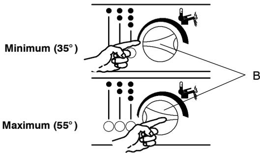
Adjustment of the DHW temperature is completely separate from that of the CH circuit.
