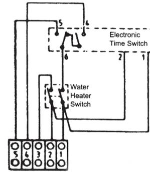
Link terminals 4 & 5 when using a single immersion heater
