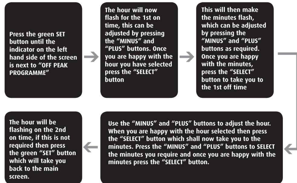
If your electricity tariff offers multiple off peak periods then the 2nd and 3rd off peak periods should be set up by repeating the above procedure. Should you not require any further off-peak settings ensure that the remaining periods are set at the same time. For example; 2nd on 12:00pm – 2nd Off 12:00pm; 3rd On 12:00pm – 3rd Off 12:00pm (These are de-fault settings).
