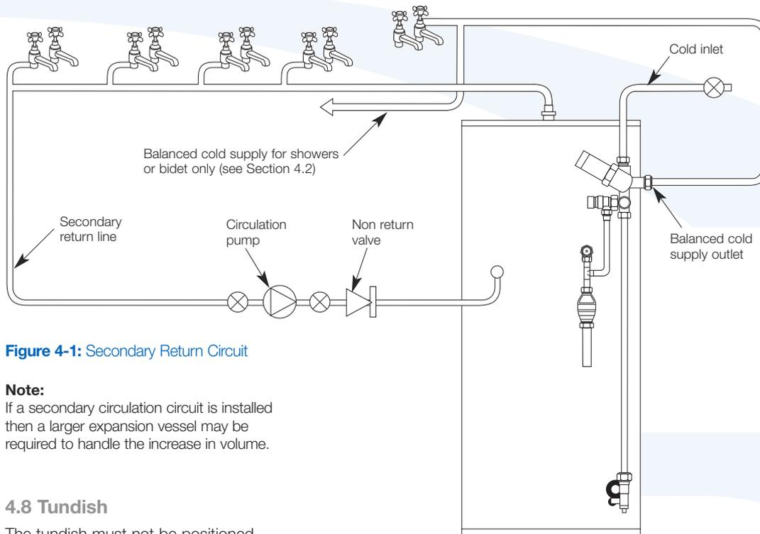
**Figure 4-1: Secondary Return Circuit**
