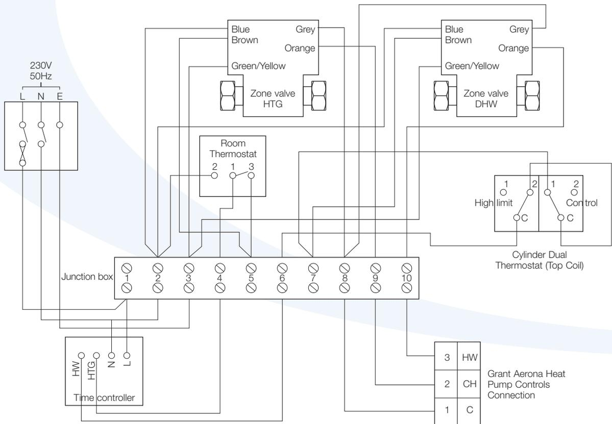
Figure 5-3: 'S' Plan wiring layout - for Grant Aeron heat pump
