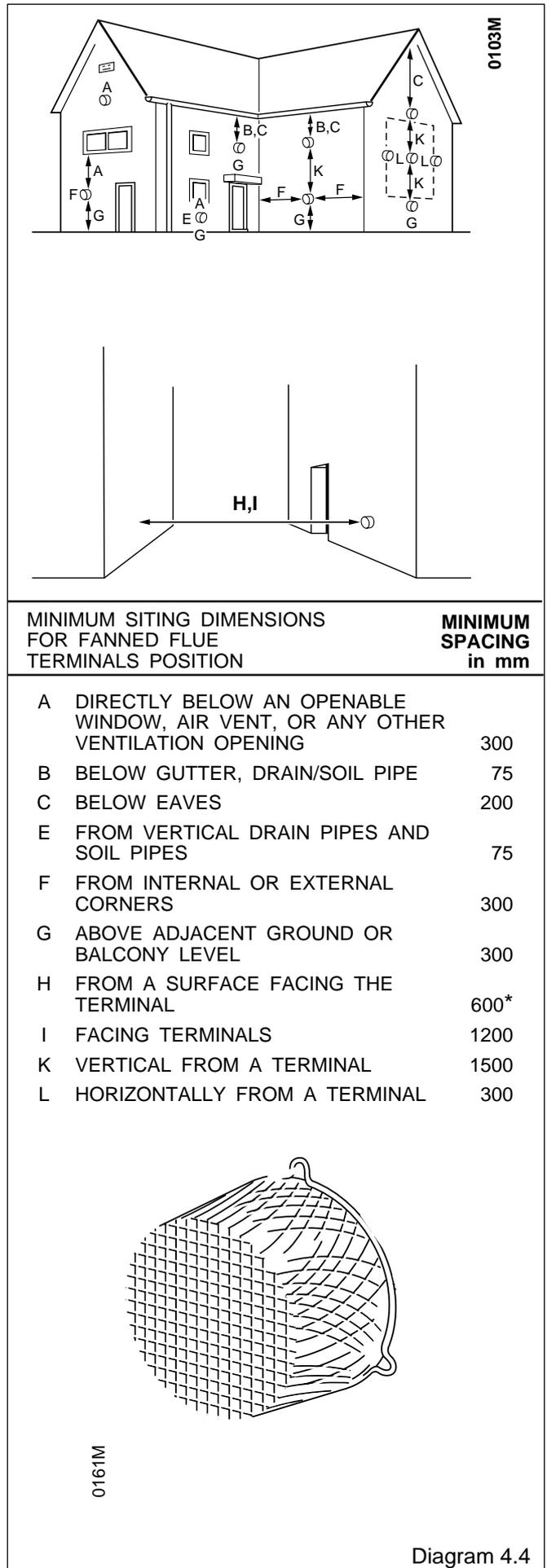
\* It may be necessary to increase this dimension to prevent staining of adjacent walls depending on weather conditions.
