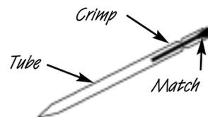
Take a length of 10mm dia pipe and seal one end. Crimp the pipe to prevent the match from sliding down inside
