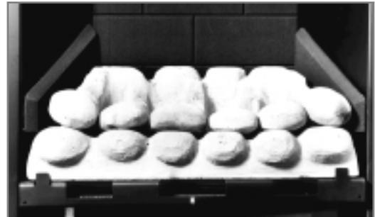
Place the front row of six pebbles on to the matrix. Ensure the pebbles are firmly against the side cheeks as shown in the photograph. If necessary, pull the pebbles forward slightly to ensure their rear edges do not overhang the flame ports. The edges of the pebbles **MUST NOT** be allowed to enter the flame ports.
