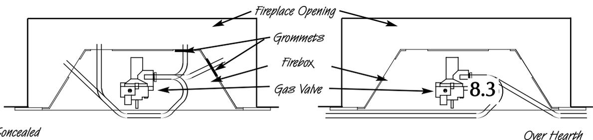
If using an across the hearth connection, then the firefront is notched and the supply pipe can be routed through this.
