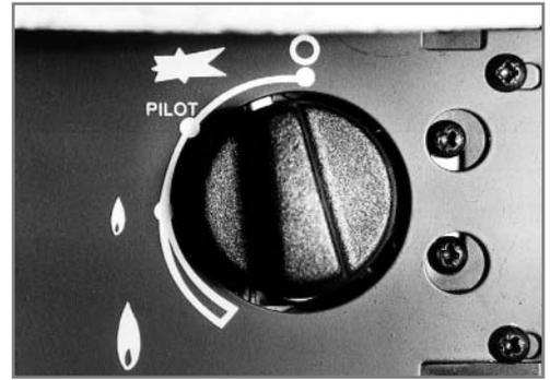
When the pilot lights after the spark, keep the knob depressed for approximately ten seconds. Now release the knob and the pilot should stay alight. If not, repeat ignition. If the pilot is extinguished *during use*, wait three minutes before repeating the ignition procedure.
