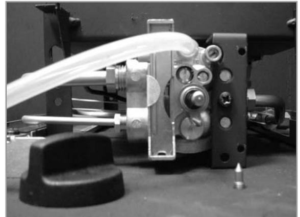
The setting pressure should be in accordance with the figures stated on page 2 of these instructions. The fire is factory set to achieve these pressures, and any significant variation could indicate a supply problem.
