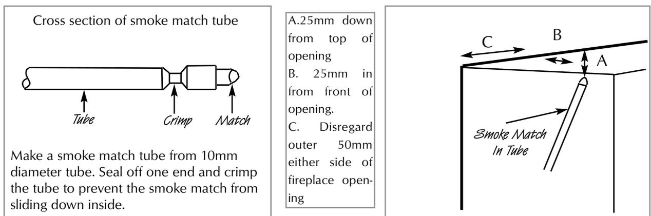
**NOTE:** If spillage is still indicated after undertaking all of the above, there may be a fault in the flue, or insufficient ventilation is present.
