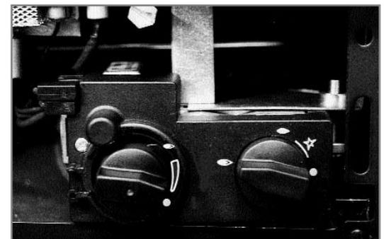
The remote control unit allows operation of the main burner setting between maximum and pilot only setting. It does not permanently turn the pilot on or off.
