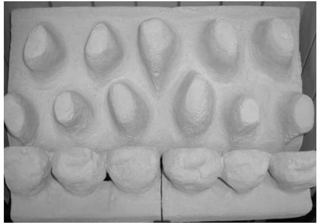
2. Open the bag of 22 ceramic pebbles. All of these pebbles are the same size. Take five pebbles and place them as shown. Care should be taken to ensure that the pebbles bridge the gap between the front strip and the six supports at the front of the matrix. Care should also be taken not to push the pebbles right down between the supports, as this can affect the flame picture when the appliance is running.
