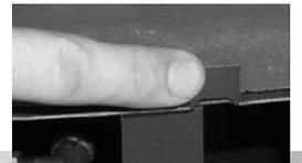
2. Next, remove the front coal strips from the protective packaging and position as shown. The rear edge of the front coal strips should fit in front of the burner rail. Again, do not place on top of the burner rails. When the front coal strips are in position bend up the three metal tags at the front of the tray to retain (inset).
