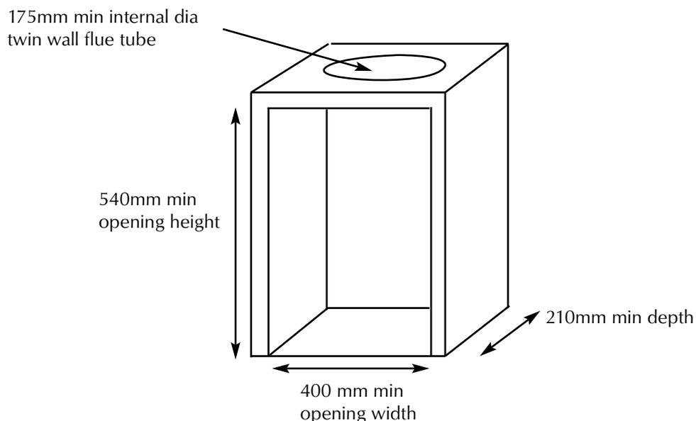
Some flue boxes may require minor adaption when fitting the fire using the cable fixing kit.
