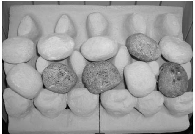
4. Now take another six pebbles and place behind the second row of coals, as shown. The pebbles may be orientated as desired to achieve a realistic effect. Keep the spacing between the pebbles even and uniform.
