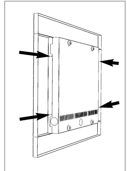
**Serenity and Saturn models;** The out casing / frame components are fitted after the main firebox has been fixed to the wall. The ceramic tiles are factory fitted.
