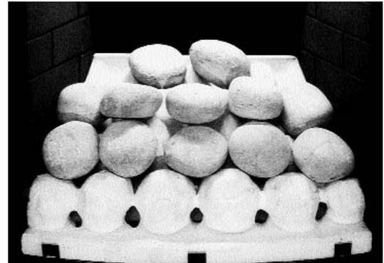
5. Finally, take the four remaining pebbles and place at the back of the fuel matrix as shown. Once again, the pebbles may be orientated as desired in order to give a realistic effect. Avoid pushing the pebbles down between the supports. The fuel bed is now complete.
