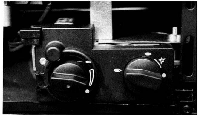
The remote control unit allows operation of the main burner between maximum and pilot only setting. It does not turn the pilot on or off.
