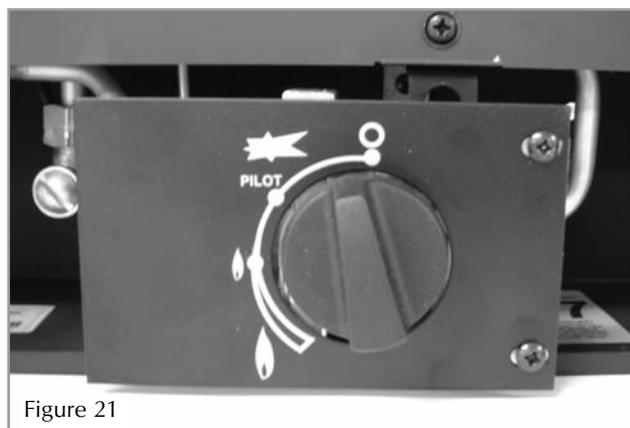
To turn to the PILOT position from the HIGH or LOW positions, press the control knob in, and return to the pilot position and release. To turn the fire off, keep the knob pressed in, return to the OFF position and release.
