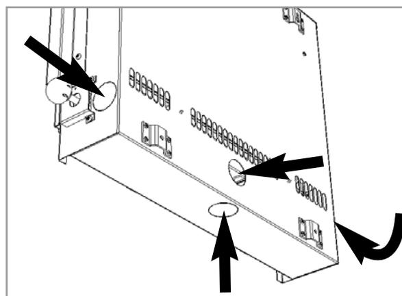
If a concealed gas connection is to be made, the supply pipe should always be sleeved through walls and floors using the shortest possible route. For concealed supply pipe routing, pipes must (where possible) be vertical and providing there is sufficient wall thickness available, they should be placed in pipe chases. Horizontal pipe runs should be avoided. Prior to chasing a solid wall, an inspection should be made to note the proximity of any cables/sockets outlets which may already be buried.
