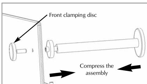
Compress the column assembly and position behind the glass panel, lining up with the appropriate hole. Release the assembly when in position and secure in place by refitting the front clamping disc.
