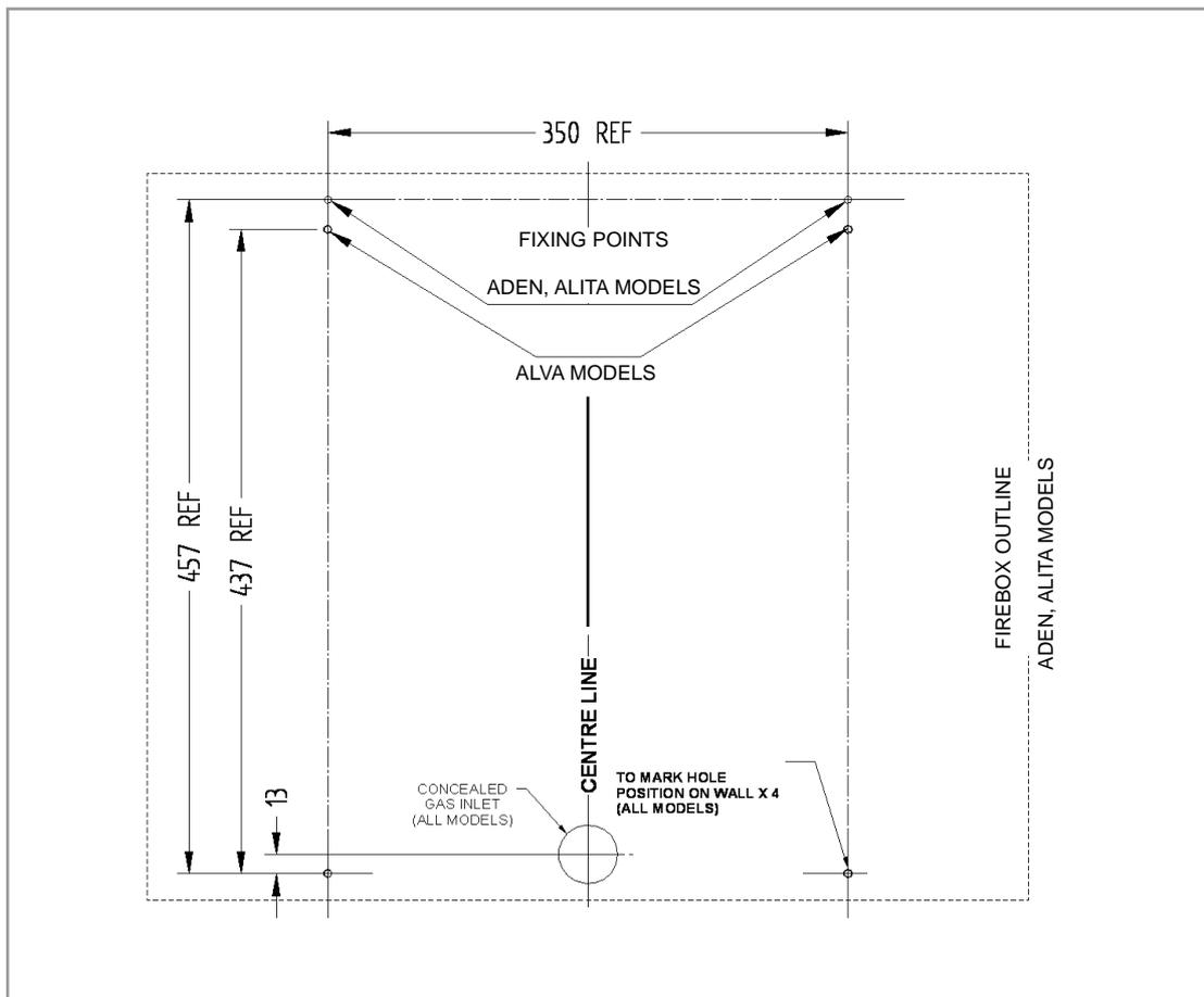
If the appliance is to be mounted on the inner leaf of a conventional cavity wall, or a solid wall, drill four holes using a 7mm masonry bit. Insert the fibre wallplugs provided.
