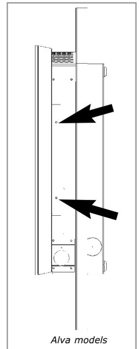
**Alva models** : The front section of the frame assembly should now be fitted. Remove the extruded frame assembly from the packaging. Position the frame onto the front of the fire, ensuring that the inside edges of the frame are pushed up to the stainless steel window frame fully. Insert four retaining screws in the positions on the side of the firebox as shown.
